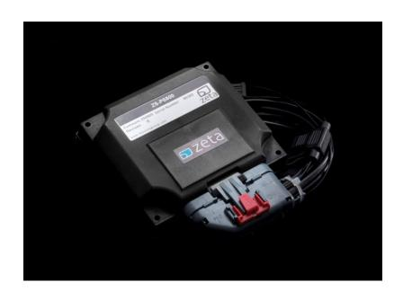
Zeta's Energy Management System (EMS) optimises the energy collection from the solar panels and manages the power in the batteries.
